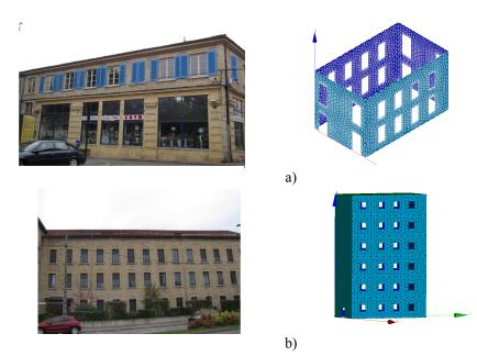
Figure 2: Example of mesh generated for different typologies of old masonry building. a) house; b) industrial building
