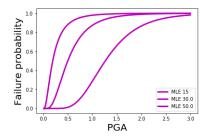
Figure 5: Fragility curve for failure mode of 15%, 30% and 50% frequency shift
