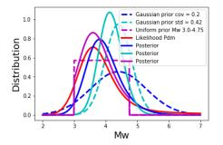
Figure 7: A priori and a posteriori magnitude a set of observation (four buildings without damage and one with light damage)
